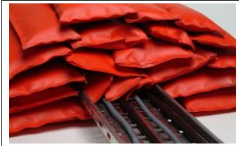
Manufactured from a hard wearing specially treated glass cloth filled with a mixture of mineral fibre and reactive expansion agents, which on exposure to heat from a fire will first expand and then harden to provide a complete and durable seal against the passage of fire, smoke and hot gases.
