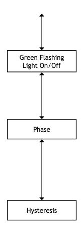
Green flashing light on / off. By using the right and left keys you can turn the green flashing LED, located on the head and controller, on or off. This is a useful way of identifying the beam head you are working with (press enter to return to mode change or down to go to phase).
