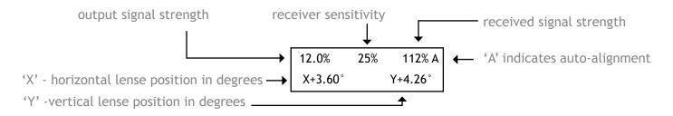
Auto alignment in 'fast' mode will take, on average, 3 minutes and in normal mode up to 30 minutes the better the beam is aligned before auto alignment (high AQ readings) the shorter the align time. Once finished **Align Complete** will appear on the screen, simply press **left back** to OK and exit.
