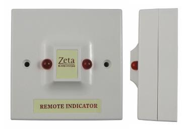
The ZTA-LE2 remote LED indicator has been designed so that it is loop powered and can be installed anywhere on the loop (it can either be connected as part of the loop, or as a spur from the detector it is indicating.). This minimises the amount of wiring from a detector to its remote indicator.
