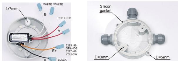
Detector mounting holes, 2x(4x7 mm) c/c = 70 mm. **E+/E-** = Ext. LED. **A/B** = zone line in/out (or end-of-line device). Connectors for wire diameter 0.6 - 1.2 mm (approx. 0.3 - 1.13 mm<sup>2</sup>).
