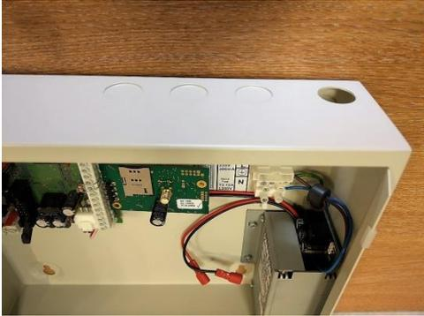
2. Unscrew the antenna cable from the mounting bracket and use a hacksaw to cut the antenna bracket 33mm from the end. (This may have been supplied pre-cut).
