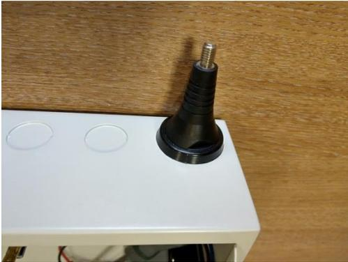
6. Screw the SMS antenna onto the base.
