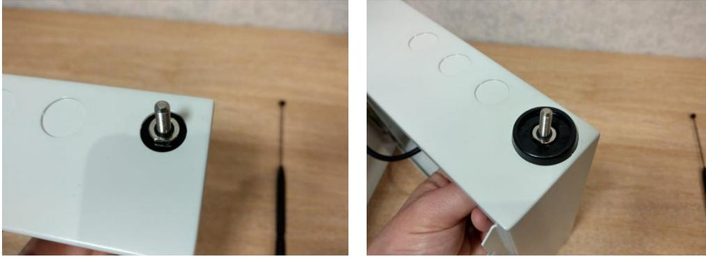
5. Mount the antenna base onto the screw.
