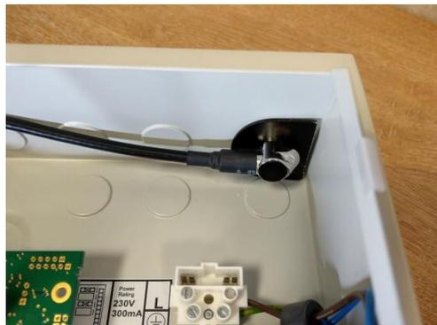
The excess sms antenna cable can be coiled up and secured with a cable tie within the panel. Alternatively, the antenna cable can be shortened for a cleaner installation. If it is not already shortened, trim the cable to 335mm and terminate it with a 50Ω SMA crimp connector (Farnell part number 170-4346).
