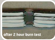
4 new enhanced FP cables
