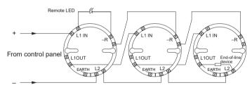
Wiring diagram of monitored Series 65 zone with common remote indicator
