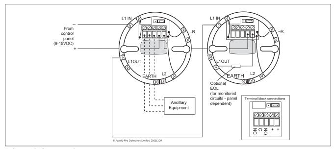
Fig.2 Typical Monitored Four Wire Security System Wiring Diagram
