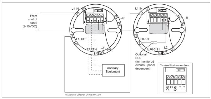
Fig.1 Typical Two Wire System Wiring Diagram
